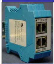
The 2C53 Ethernet 10/100 Base-T(X) Unmanaged Switch Module requires little or no user configuration. The data rate is automatically negotiated and the ports will auto-sense Full or Half duplex operation. The 2C53 will automatically learn the addresses of the devices connected to each port (up to 1024) and will buffer and route messages accordingly.
